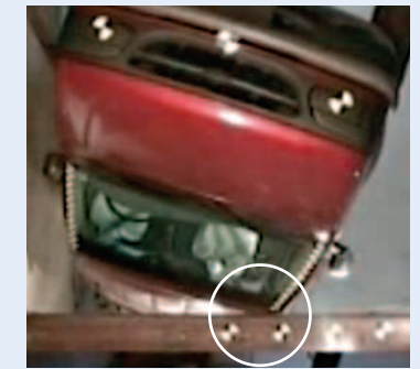
Dynamic tests clearly showed the roof defect.
